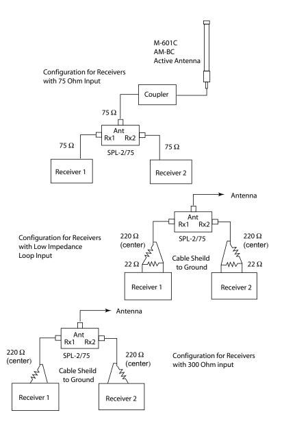
**In combiner configuration**, two different antennas may be used to feed one broadband receiver. Shown below are two suggested antenna configurations that may be used with the SPL-2/75.
